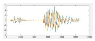
The PPV from the cast that was shot with the signature hole was 1.24 IPS at the well. The distance from the well was 2,000 feet. The delay timing sequence was chosen by DynoConsult.
